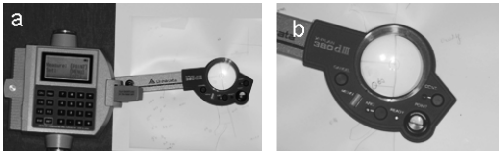
Figure 5. (a) Digital planimeter. (b) Measurement of the areas using a digital planimeter.
