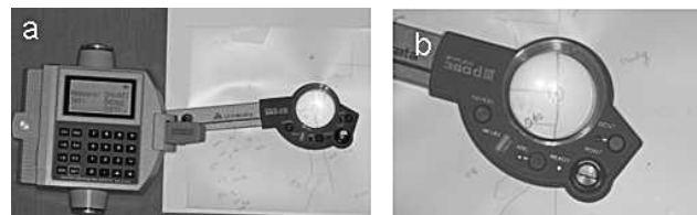
Figure 5. (a) Digital planimeter. (b) Measurement of the areas using a digital planimeter.
